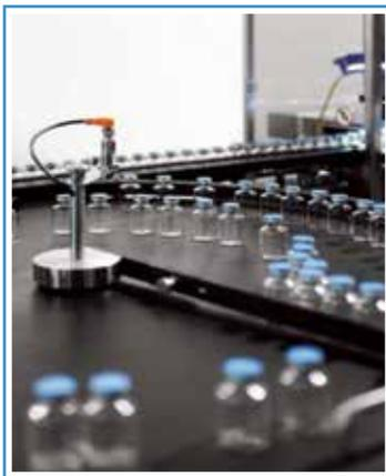
Rotary accumulating and transfer tables
