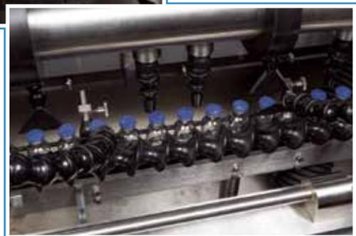
As a stand-alone system, the EVW can be equipped with a rotary infeed disk with loading platform. Machine above shown with an extended drying section for high throughput requirements.
